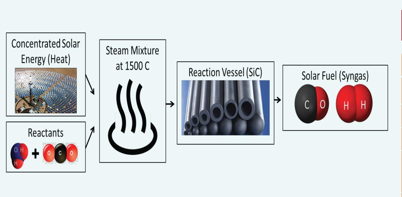
Enable solar fuel reactors in 1500°C steam - need high temp. components such as SiC
